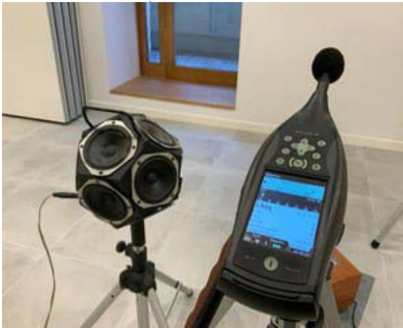
Some of the tools used to assess noise levels and Sound Transmission Class (STC) ratings of assemblies.
